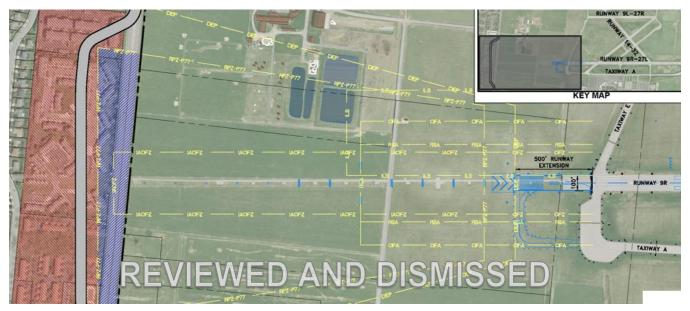
**Note:** Light blue lines indicate the proposed runway extension, yellow lines show various required airport zones, purple-blue shaded areas show runway protection zones (impacted properties), and red shaded areas would impact the existing road network and relocation of both Godown and Sawmill Road.
